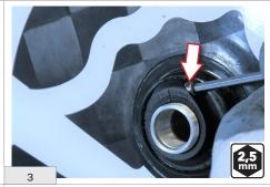
Undo the locking screw for the play adjustment ring nut.
