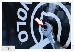
Screw the left end to a torque of 11/11.5 Nm using a 18
