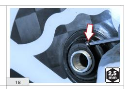
Tighten the play adjustment ring nut screw to a torque of  ${\bf 1.5~Nm}.$
