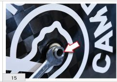
Lock the axle on the right-hand side using a 15 mm fixed wrench.
