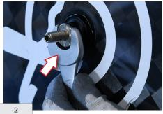
Unscrew the left end using a 17 mm fixed wrench.
