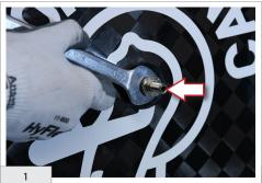
Lock the axle on the right-hand side, using a 14 mm fixed wrench.  $\,$
