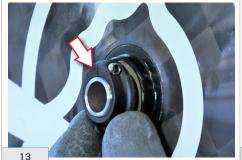
Screw the play adjustment ring nut back on.
