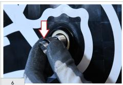
Remove the cone pusher and the cone.
