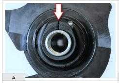
In order to unscrew the ring nut, undo the screw until a slot is visible between the two edges of the ring nut itself.
